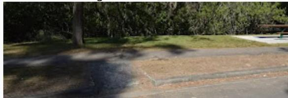
There is a single ramp to access the path from the car park. The concrete ramp is 1.2m wide. The ramp is in a marked parking bay and may be blocked by a car.
