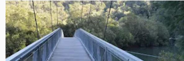
The bridge over Cockle Creek is 1.8m wide, has 1m high handrail and a timber decking. The steepest section is 5.3° (1:10 or 9.2% grade). The bridge is 40m long.
